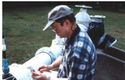
Figure 25 – Sampling MUD Well-Casing Headspace and Groundwater (Campbell, Campbell and Saribudak, 2004)
