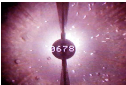
Figure 28 – Minor Natural Gas Bubbles Rising in MUD Well Casing at Depth 678 Feet (From Campbell and Wise, 2013)
