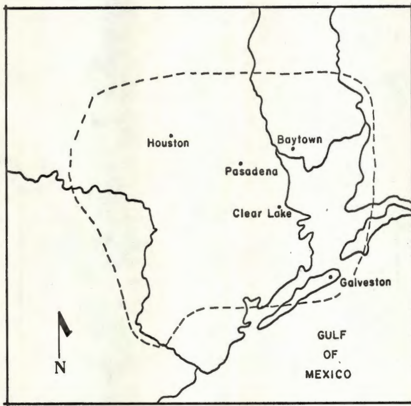
Figure 1. Approximate 3,000 square miles (within dashed line) affected by land surface subsidence in the Texas Gulf Coast area.
